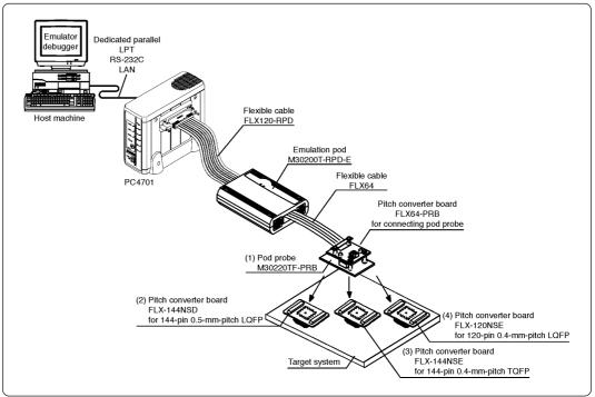
Figure 2.1 System configuration
